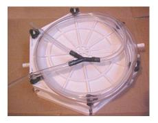
Allow the filtering plates to soak in water for a few minutes. Make sure the intermediate ring is nicely in the middle. The nuts and bolts are then fitted and tightened. Remember that the nuts must all be equally tightened, so we alternatively tighten two on each side. Connect the outlet of the container to the filter inlet (separator) using a PVC hose. Fill the container with water to a maximum of the 11.4 litre mark, screw the pump on it and start pumping.
