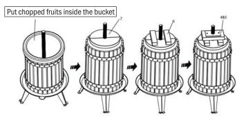
Place the nylon washer (3) on top of the pressure plate assembly as shown in the illustration. Screw on the trunnion (2), push the handle into the trunnion and rotate the handle (1) down to press the fruit down into the barrel.
