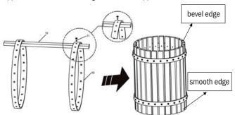
Wooden pressing plate (5) and metal pressing plate (4) assembly with screws (11).
