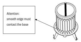
5. Put the empty juice bag (9) in the press with the threaded rod (8) through the hole in the juice bag. Stretch the juice bag over the bucket. Then fill it with the chopped fruit and, if necessary press down the fruit by hand. When the juice bag is filled, fold it inwards.
