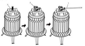
8. Never use an extension bar on the handle. The second pair of blocks provided may be inserted when space allows for it, to force the wooden plates as near as possible to the base of the press. If the handle reaches the wooden barrel assembly and pressure still needs to be increased, release the trunnion and place one set of wooden blocks between the wooden plates and the pressing plates. Place a container beneath the outlet spout in the base (13) to collect the juice.
