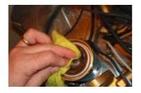
The pump casing should also be cleaned. Then put the cleaned rotor ball back into the casing.
