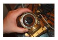
The rotor ball is now visible inside the pump. **Caution:** Rotor ball can fall out! Damage to the rotor blades will lead to subsequent failure of the pump!
