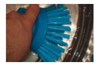
Pour water up to approx.  $2\ cm$  above the heating coil and heat it manually to ~35 °C using the control unit. Attention: The pump must be vented by switching it on and off several times! Then disconnect the Braumeister from the power supply again! Now brewing residues can be removed from the inside of the container and the heating coil with a brush, preferably directly after each brew.
