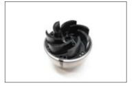
The rotor ball is removed from the housing for cleaning. Any brewing residues must not clog the holes and must therefore be removed carefully.
