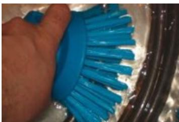
Pour water up to approx. 2 cm above the heating coil and heat it manually to ~35 °C using the control unit. Attention: The pump must be vented by switching it on and off several times! **Then disconnect the Braumeister from the power supply again!** Now brewing residues can be removed from the inside of the container and the heating coil with a brush, preferably directly after each brew.
