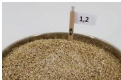
Clearance of 1.2 mm; clearly too finely grinded.
