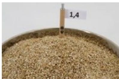
Clearance of 1.4 mm; not yet completely optimal.
