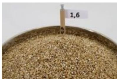
Ideally with a clearance of 1.6 mm; suitably grinded. If whole grains do not break when pressed on, the grain has been too coarsely grinded.
